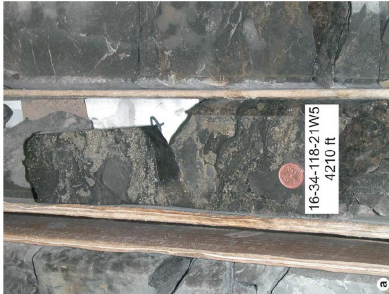
Figure 22. Sulphide-cemented carbonate breccia in core from northern Alberta. a. Sphalerite, pyrite and minor galena in brecciated Keg River Formation from drillhole 16-34-118-21W5, above the magnetic trace of the Great Slave Shear Zone. b. Pyrite- (and sphalerite?) cemented carbonate breccia from the Jean Marie Formation in the depth interval 252–267 m in drillhole 04-03-100-07W5, north of Birch Mountains.
